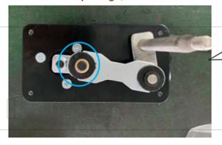
Remove snap rings / washers by circlip plier, and take this assembly off
