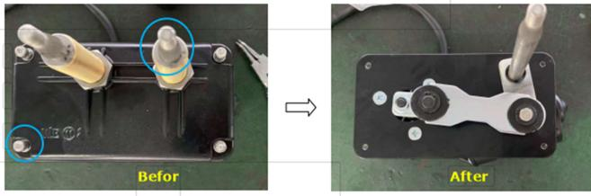
2. Remove snap rings/washers form link rod:
